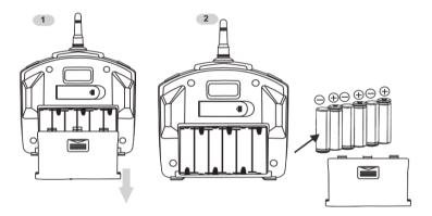
Insert the battery by sliding the cover down. Then insert 6 x AA batteries as indicated under the cover.
