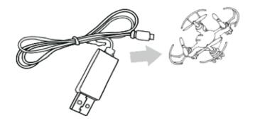
Plug the USB into a USB socket and connect the copter to the charger. This can only be done in one way: by firmly connecting the charging cable.
