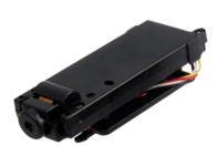
This model can be equipped with a camera. If your model doesn't include it, you can find it from your retailer or on www.wltoys.eu. The camera is installed as explained under module. You can install the SD card by pushing it in the rear slot until you hear a click. To take out, press again till it is pushed out.
