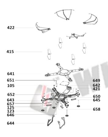
Description | Quant Ref 105 | Bearing | 8 123 | Gear | 4 125 | Main shaft | 4 415 | Blades | 4 421 | Battery | 1 422 | Protect part | 4 641 | Upper canopy | 1 6 642 | Battery cover | 1 643 | Lower canopy | 1 644 | Landing skid | 2 645 | Lamp cover | 4 646 | Back lamp cover | 1 649 | PCB | 1 650 | Red light | 2 651 | Motor clockwise | 2 652 | Motor counterclockwise | 2 657 | Green light | 2 658 | Indicator light | 1
