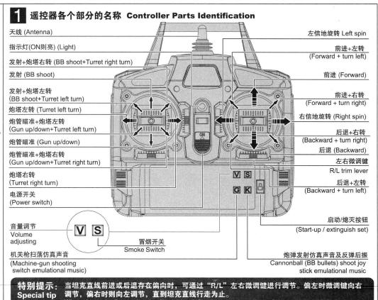
When the tanks forward or backward be deflection, can be adjusted through the "R/L" left and right
