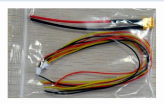
LAN-to-4Pin wire*1 (used for module parameters setting)
