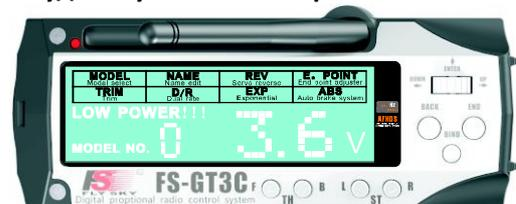
Following screen will be showed when the voltage is lower than 3.7V .
