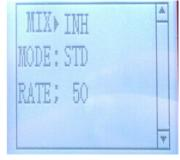
4.Press the button key Enter, the value stops flashing, the setting is finished now.5."Mode"and "Rate" can also be set by the same step.6. Press button key Evit to be back to initial across
