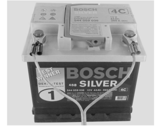
Using terminal clip attaching to car battery
