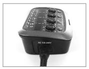
3. When the charger is powered on, 4 status LEDs will blink once with one beep and all 4-digital LED Indicators will display 8888. After that, 4 LEDs will extinguish and all 4-digital LED Indicators will display the charging current which indicates the charger is ready to charge.
