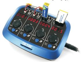
7. When the charging process is finished, the status LED turn green and blinks 5 times with audible sound. And the status LED stays green and the 4-digital LED will display "FULL".
