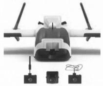
KIT Includes only airframe. (Motor, ESC, Servos, Propeller, ZOHD VC400 Camera, ZOHD Kopilot Lite, Battery, Radio controller, Charger are not included.)
