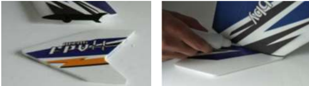
5.Connect the fuselage and wing with two pieces of stainless latch pipe, and fix with rubber band.
