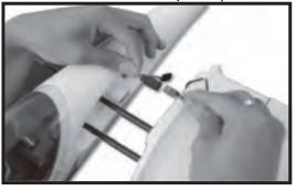
12. Put the metal joiners through the corresponding hole of the fuselage and connect the servo wires of the ailerons and flaps.
