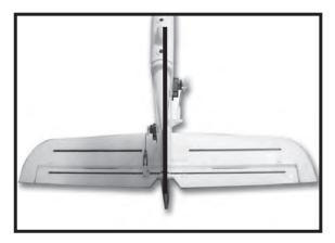
Also, we strongly recommend installing the included 'clevis keepers' to provide added security for the clevises. Typically you can carefully slide the keepers over the clevises when they are not connected to the control horn. Then, after connecting the clevis to the control horn and 'snapping' the clevis together you can slide the keepers into a position that does not allow them to 'bind'against the control horn during movement of the surface.
