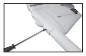
5. Install the fin to the fuselage with the screw provided.
