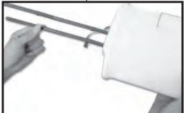
11. Insert the metal wing joiners to the main wing.
